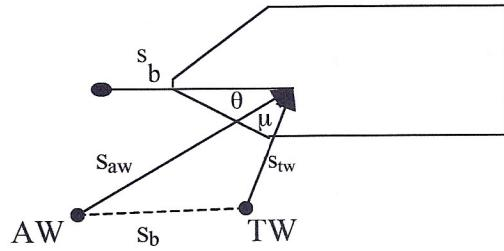
Forward wind (FW) coming from directly ahead at boat speed  $s_b$
